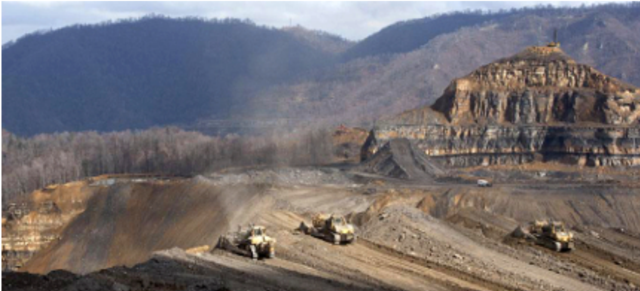
Mountaintop-removal and valley-fill coal mining at Massey Energy's Edwight site in Sundial, West Virginia. (photo: Antrim Caskey)
